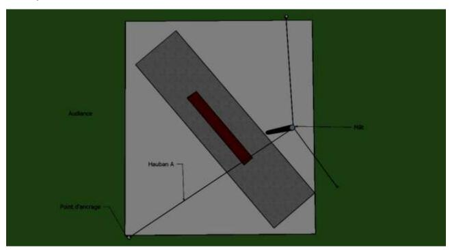
The guidewire A must be perpendicular to the teeter board. It is not obliged to anchor guidewire A to the floor; depending on the height and length with the Chinese pole the angle may vary, this does not cause any problems. The depth of the stage may also vary. Please send us the technical plans of the venue in order to allow us to properly assess the venue and make accurate measurements.
